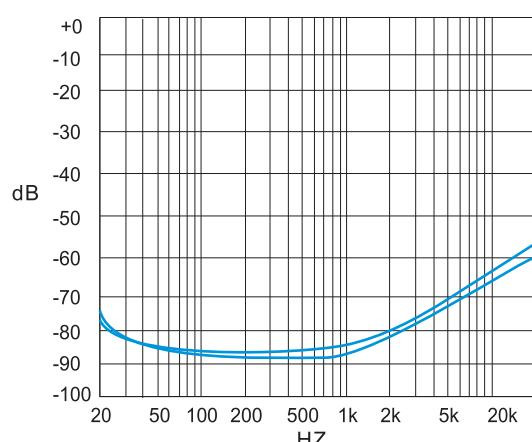
Figure 19. PSRR vs. Freq
