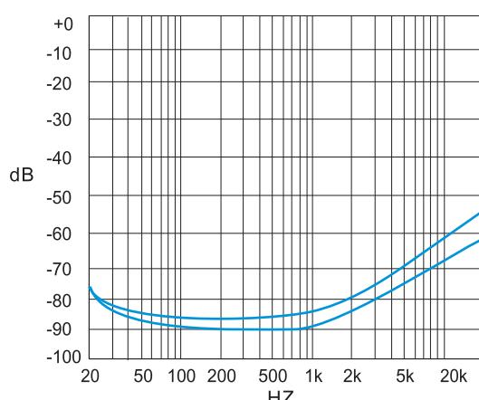
Figure 20. PSRR vs. Freq
