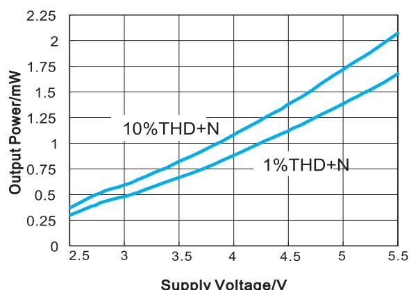
Figure 30. Output Power vs. Power Supply
