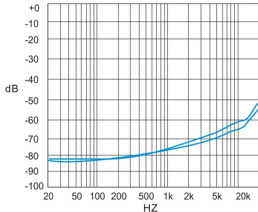
Figure 15. PSRR vs. Freq
