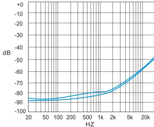
Figure 16. PSRR vs. Freq
