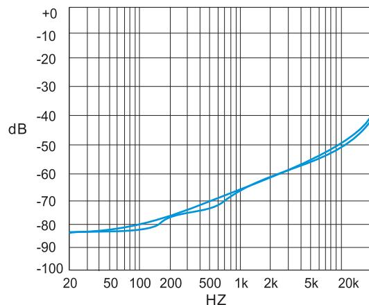
Figure 17. PSRR vs. Freq
