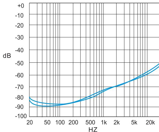
Figure 18. PSRR vs. Freq
